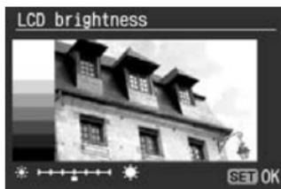
When checking the exposure of an image, prevent the ambient light from affecting the reviewed image. Also, setting the LCD monitor brightness at the center of the adjustment scale is recommended.
