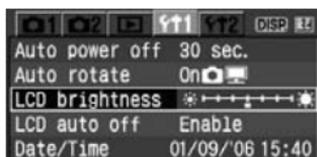
Under the [fT1] tab, select [LCD brightness], then press <SET>. With the adjustment screen displayed, press the <◀▶> key to adjust the brightness, then press <SET>.
