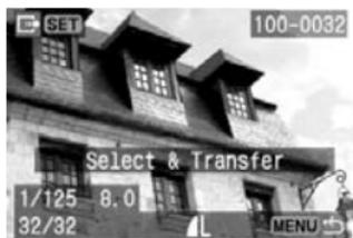
Press the <◀▶> key to select images one by one to be transferred to the personal computer. To exit, press the <MENU> button.
